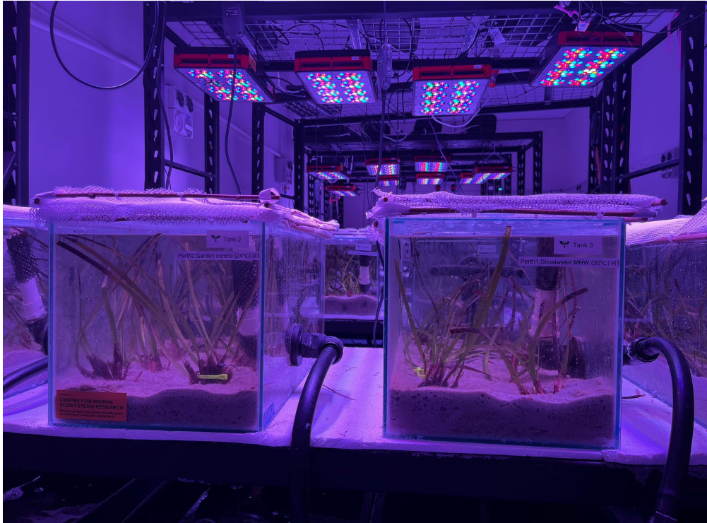
Figure 2: Posidonia sinuosa planted in aquarium tanks to test the effects of temperature and duration on the resilience of three different P. sinuosa populations: Shoalwater, Garden Island and Jurien Bay.
