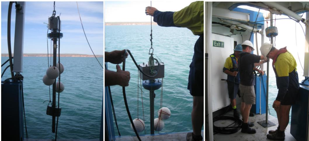
Figure 2.1. Coring method using a Vibecore-D (Speciality Products, USA) weighted vibrating head lowered from the CTD winch on the RV Solander.
