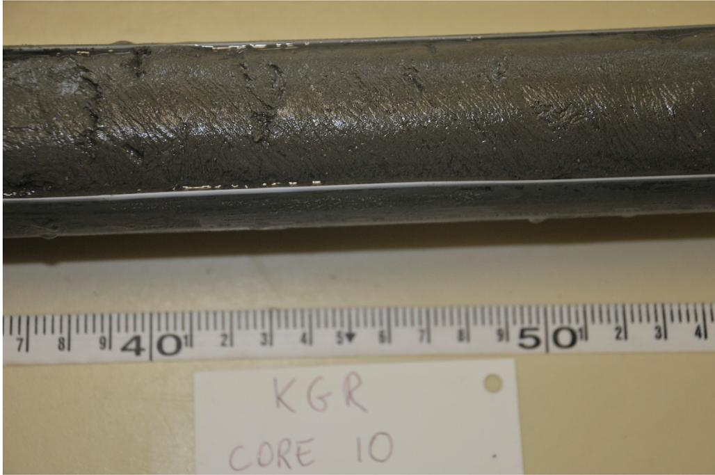
Figure 2.2. Close-up of sediment core prior to sectioning.
