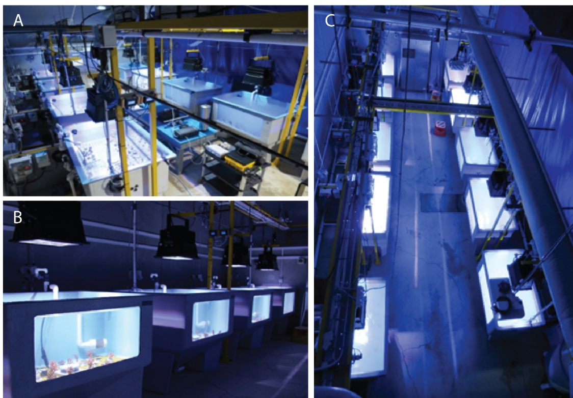
Figure 2. Images of the 10 × 1500 L tanks used in the longer-term sediment dosing experiments. Each tank received filtered (0.4 µm) seawater at 27 °C at a rate of 1 L min -1 . Water movement within each tank was controlled using submersible pumps controlled by a programmable logic controller (PLC). Each tank automatically received pulses of elevated SSCs from a concentrated 500 L reservoir via solenoid valves connected to a PLC. Turbidity, light and sediment deposition rates were recorded continuously by the PLC.
