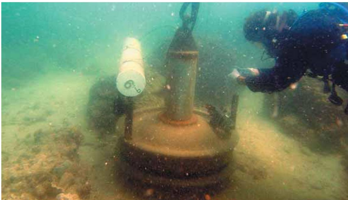
*The work team checks the instrument on a telemetered water quality logger.*
