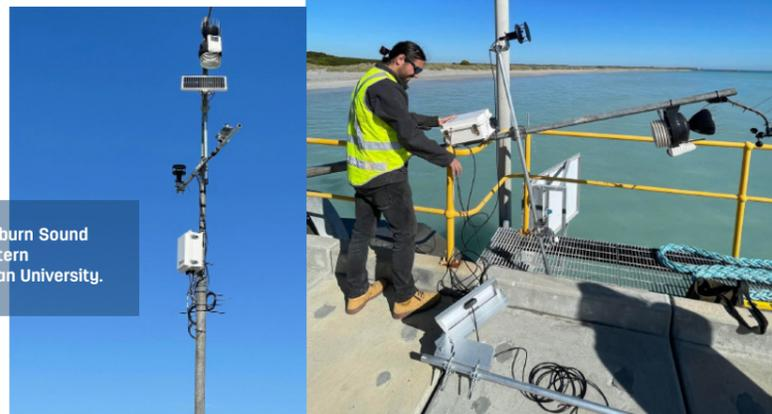
The weather station will be deployed for 12 months and measure wind speed and direction, air temperature, humidity, air pressure, solar radiation, precipitation and photosynthetically active radiation (PAR) at five-minute intervals.
