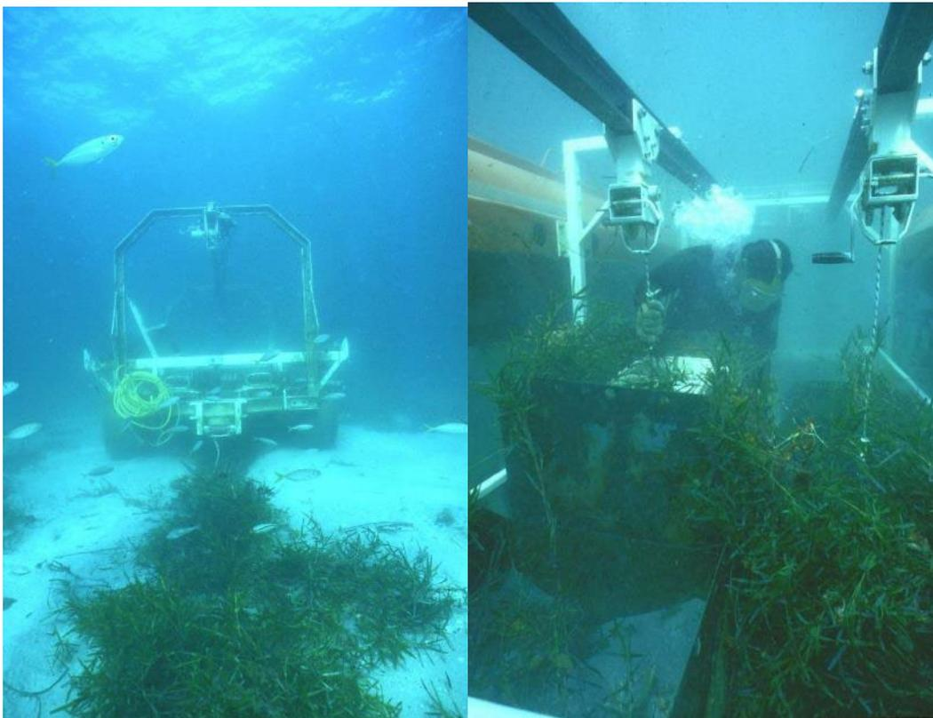
*Figure 4: ECOSUB 2 was an example of mechanising and industrialising seagrass restoration and rehabilitation. Top image shows the harvester (front) and planting unit (back) on a truck trailer. Bottom left shows the planting unit and a line of transplanted sods. Bottom right shows the shuttle unit and sods being placed into the planting unit.*
