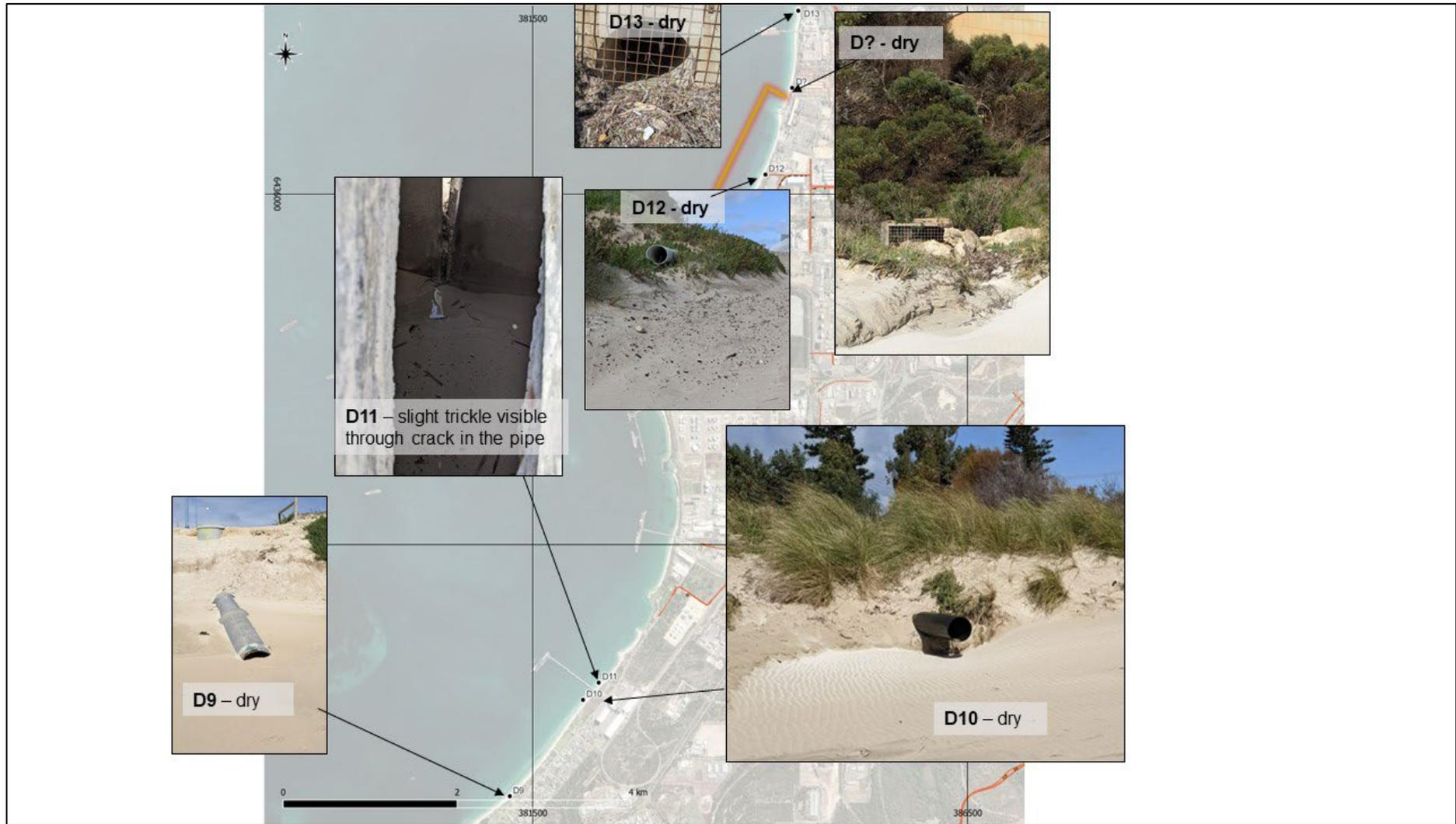
**Figure 6.** Stormwater drains D9 through D13 re-visited on 14 September 2022. Compare with Figure 4, which was during wetter conditions.
