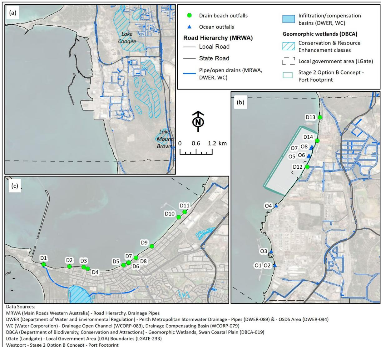
**Figure 2** Local government and main roads drainage infrastructure (a) City of Cockburn, (b) City of Kwinana and (c) City of Rockingham. The location of eight ocean outfalls identified from DWER licence documents for industries in this area and 14 stormwater drains identified during field trips (September 2022). D10 and D11 are used by CBH; D12 is used by Water Corporation (Perth Seawater Desalination Plant); D13 is 50 m from Alcoa property. D14 is an unconfirmed drain near Alcoa property.
