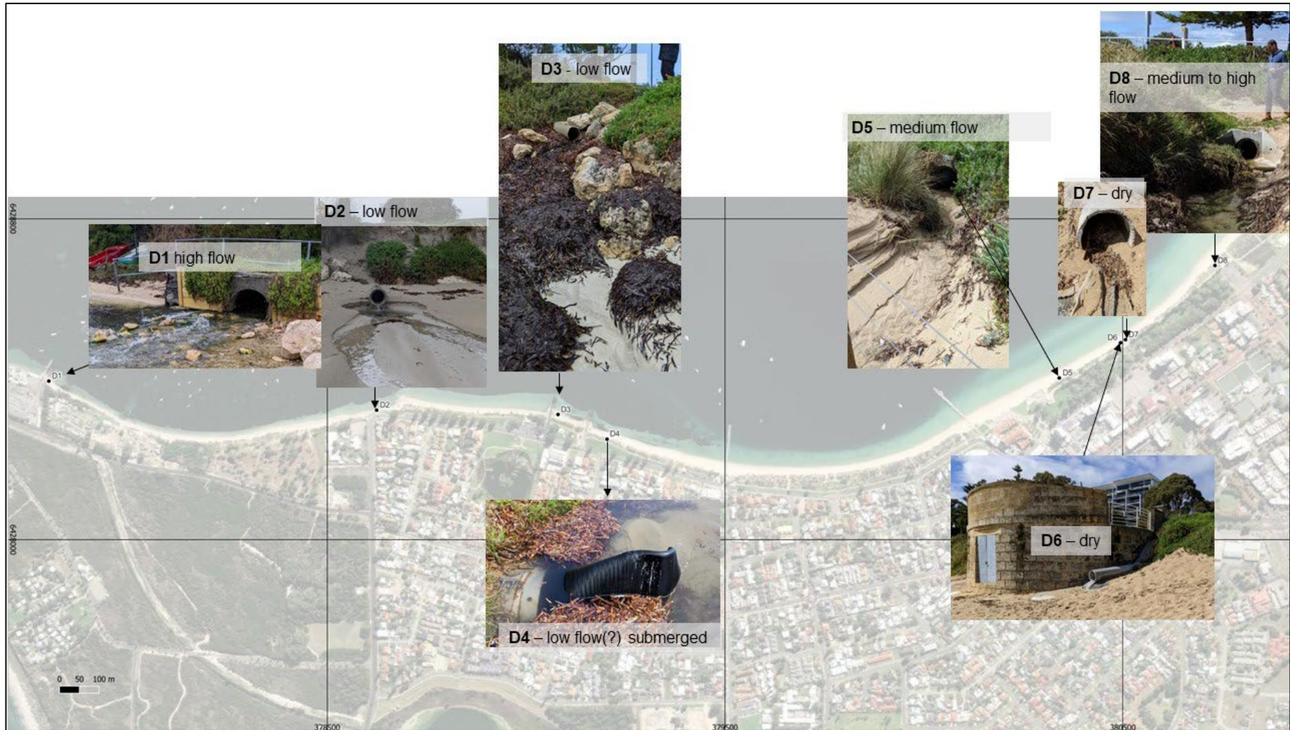
**Figure 3.** Locations of stormwater drains D1 through D8 identified during trip on 06 September 2022. These drains are all in the City of Rockingham.
