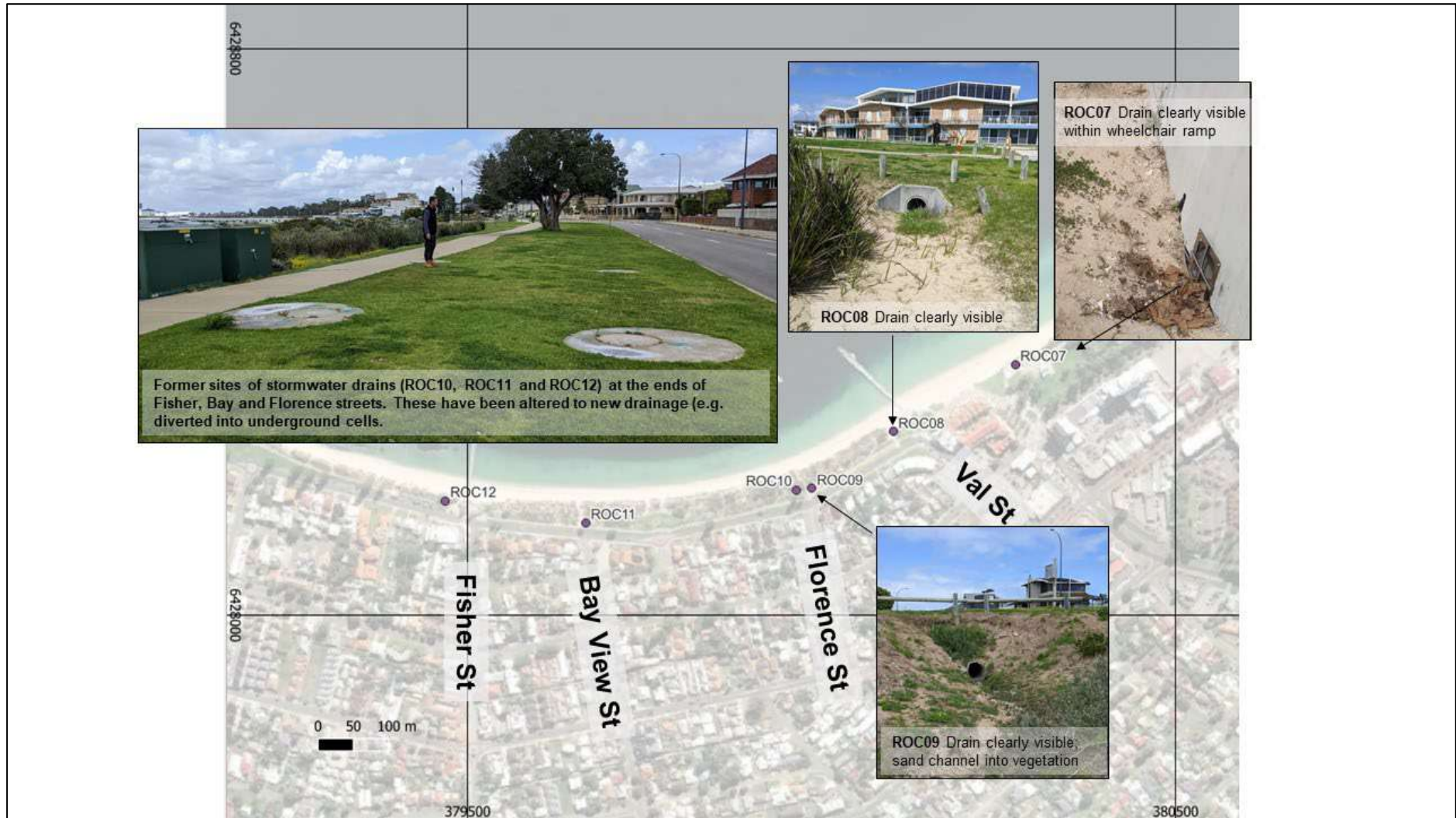
Figure 7. Drains located farther away from the shoreline and closer to roadways in the City of Rockingham, including unlined sumps in dune vegetation (photos from 14 September 2022).
