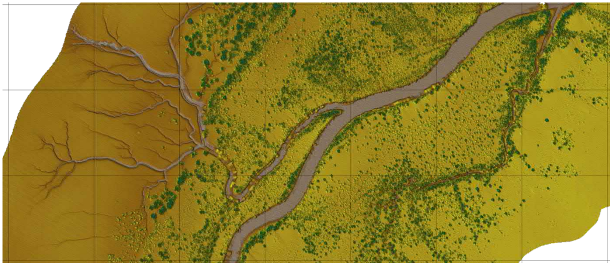
Figure 4: Exemplar LiDAR data showing Urala Creek (NE Exmouth Gulf). Grid cells = 100 m and pixel resolution is 25 cm. Green is representative of mangrove canopy.
