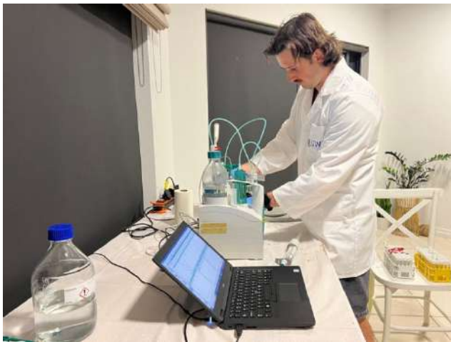
Figure 5. Alkalinity measurements at the on-site laboratory.
