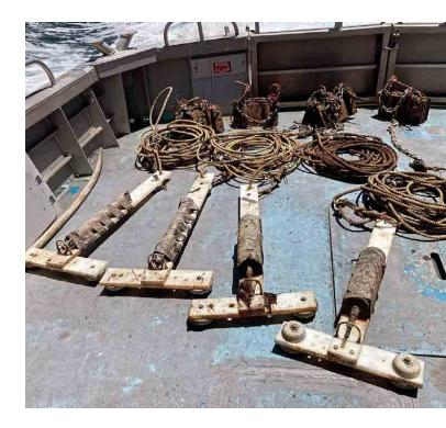
Because of the boating and fishing activity in Cockburn Sound the team decided not to attach the devices to floats which would increase the possibility of ropes becoming snagged in propellers.
