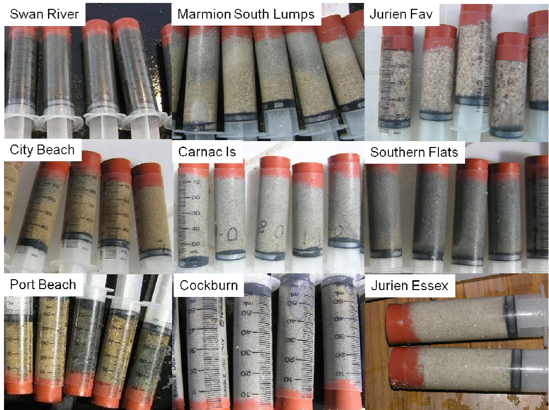
Figure 4.8. Examples of the range of appearance of sediments sampled ranging from coarse to fine sands and high and low organic loads.
