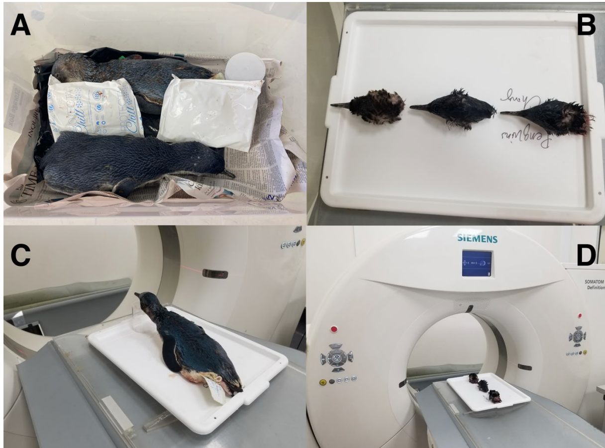
Figure 1. X-ray computed tomography scanning of the little penguins. (A) Two collected little penguin specimens (full body). (B) Three collected little penguin heads. (C) XCT scan of one of the penguins, focusing on its head. (D) XCT scan of the three penguin heads.
