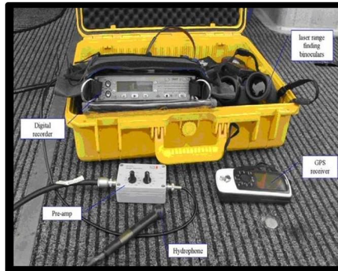
**Figure 2.5.** Hand-held recording system used for in-situ, vessel-based recordings.
