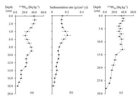
Figure 4.4. Profiles of  ${}^{210}Pb_{ex}$  and sedimentation rates at KGR2 (a, b), and  ${}^{210}Pb_{ex}$  at KGR3 (c) (error bars denote standard deviation).
