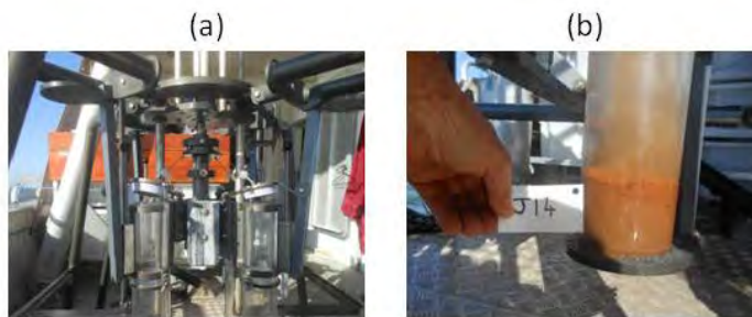
Figure 7. (a) Piston corer on deck, loaded and ready for deployment and (b) a typical core sample
