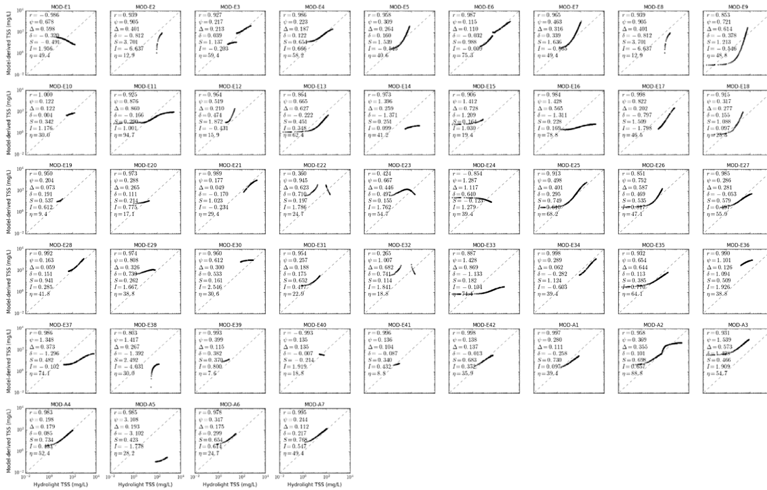
Figure S1.9. Scatter plot of MODIS TSS models in CLASS-I water for calcareous sand sediment, b_b/b ratio of 0.1, solar zenith angle of 30°.
