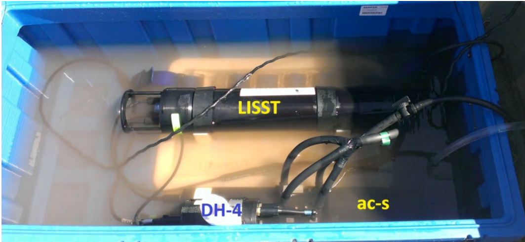
Figure 6. The ac-s as it was deployed during the field work campaign in October, 2013. The ac-s is connected serially with the LISST. The DH-4 is a submersible data logger compatible with Wet labs instruments.
