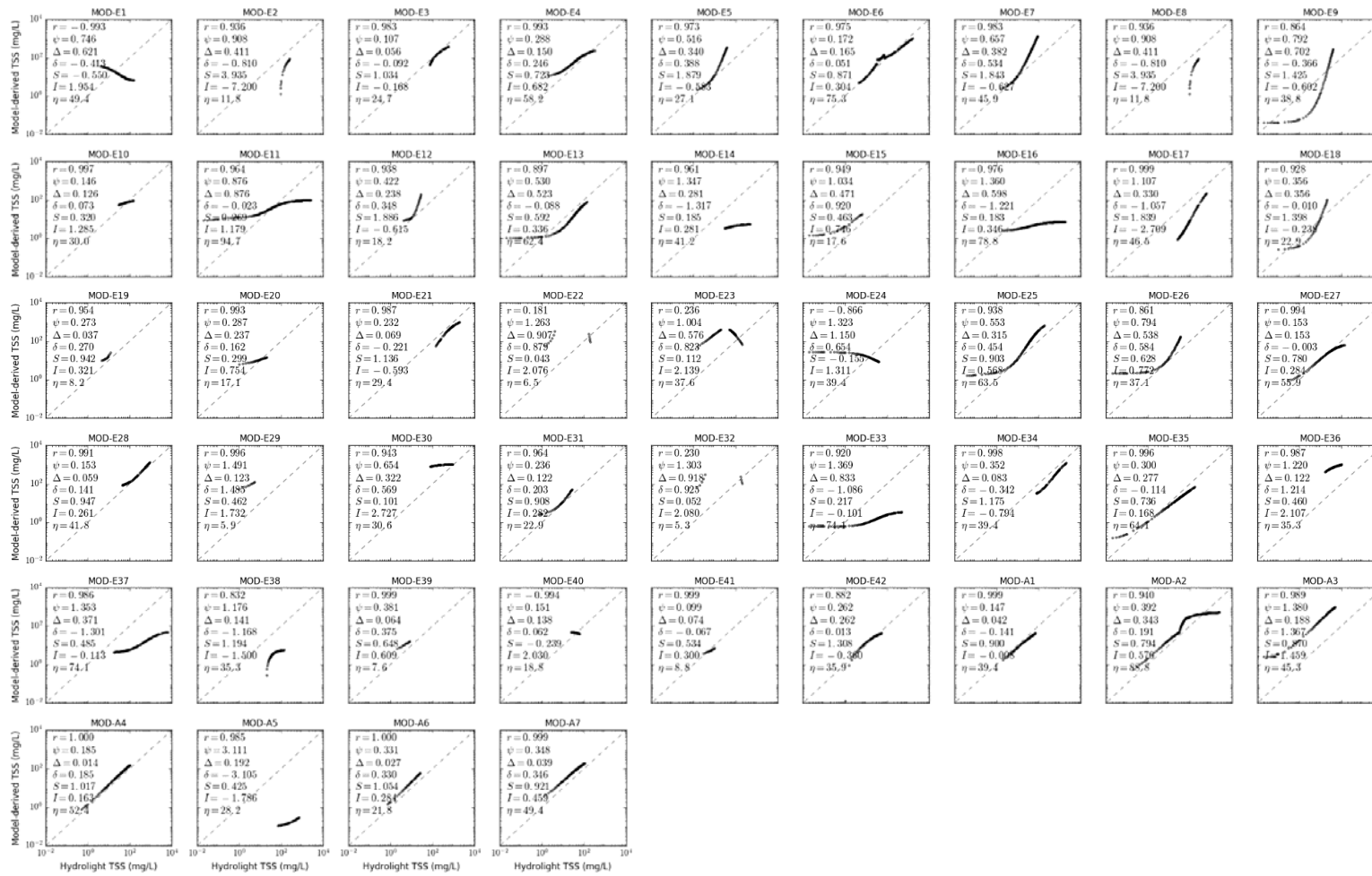
Figure S2.3. Scatter plot of MODIS TSS models in CLASS-II water for calcareous sand sediment, b_b/b ratio of 0.018, solar zenith angle of 30°.
