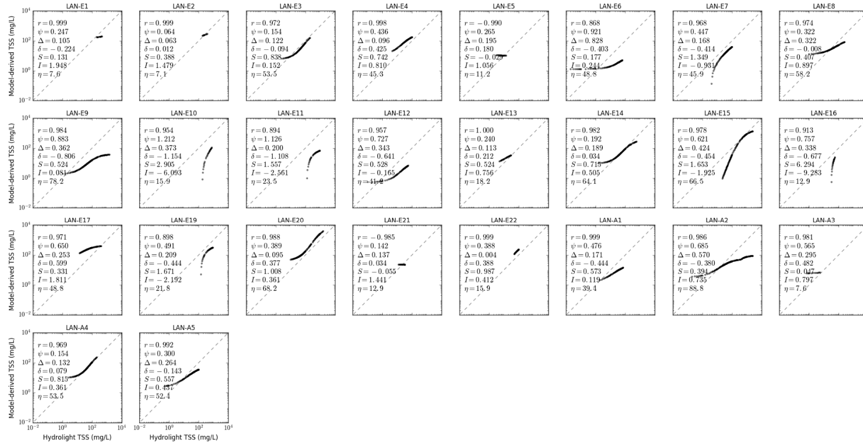
Figure S8.1. Scatter plot of LANDSAT TSS models in CLASS-III water for brown earth sediment, b_b/b ratio of 0.018, solar zenith angle of 30^\circ .
