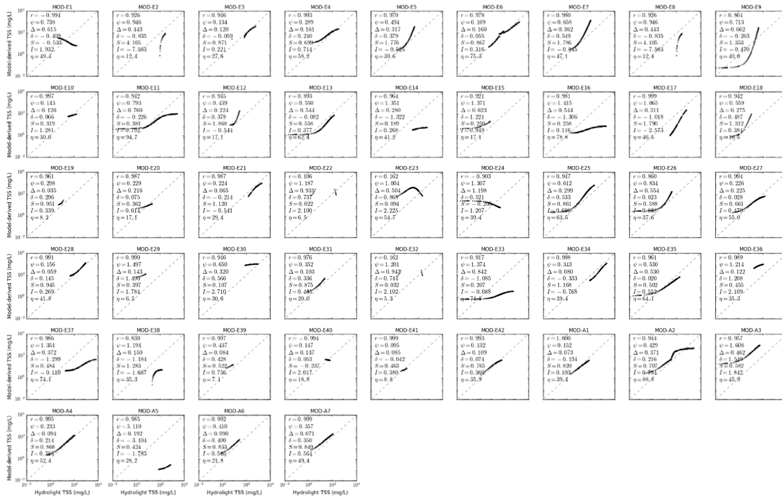
Figure S5.9. Scatter plot of MODIS TSS models in CLASS-V water for calcareous sand sediment, b_b/b ratio of 0.1, solar zenith angle of 30°.
