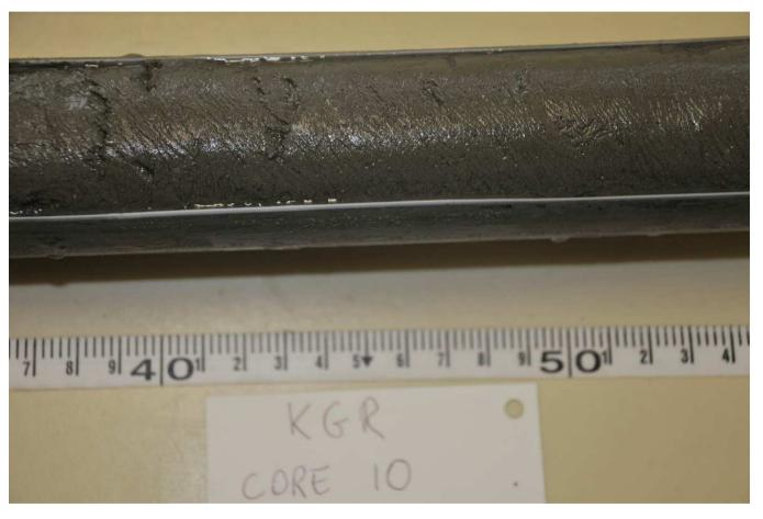
Close-up of sediment core prior to sectioning into 1 cm pieces
