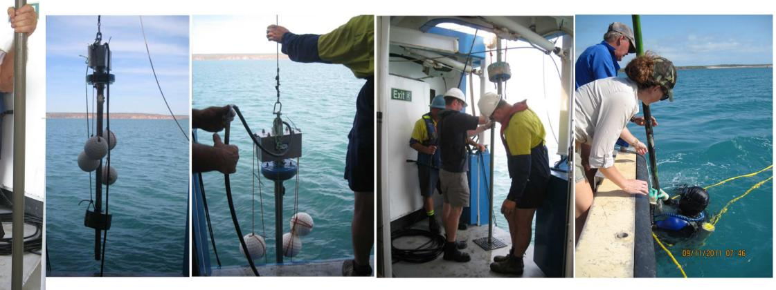
Left three panels showing coring method using a Vibecore-D (Speciality Products, USA) weighted vibrating head lowered from the CTD winch on the RV Solander, and right panel showing diver recovering a core from Cygnet Bay
