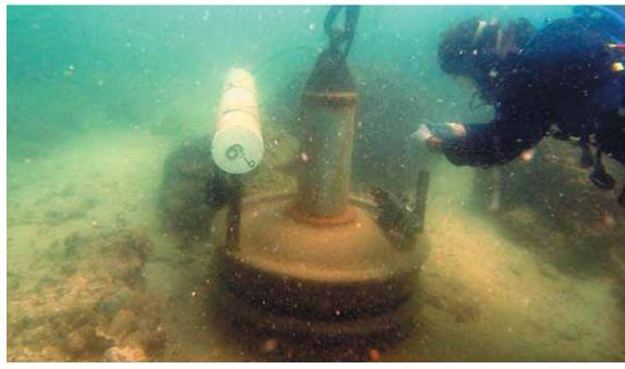
The work team checks the instrument on a telemetered water quality logger.
